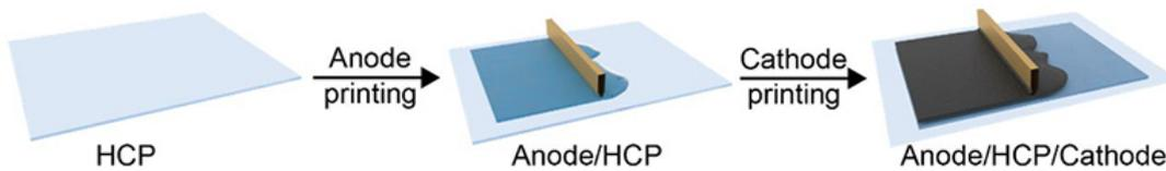
The battery consists of cellulose paper that the researchers have permeated with a hydrogel to strengthen it. They then screen print the electrodes onto either side of the cellulose paper, with the anode ink consisting of zinc and a type of conductive carbon, and the cathode containing either manganese or nickel. Finally, the researchers coat the electrodes with gold foil to increase their conductivity.
